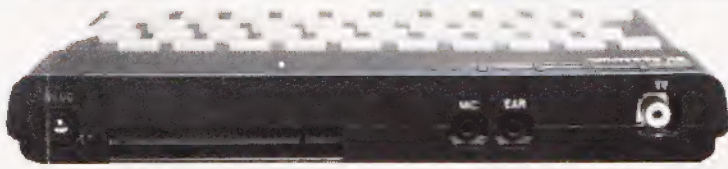
Above: The rear panel of the ZX Spectrum carries all the I/O connections. Note that the bus connector is bigger than the one on the ZX81. Below: The internal layout is very neat; the standard 16K RAM is at the bottom left. Note the two IC sockets towards the top of the case — this is where the RAM expansion sits on a daughter board.
